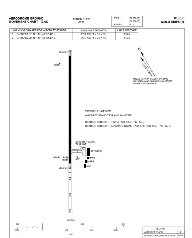
CHANGES: ADD BAR SCALE AIRCRAFT TYPE PAVEMENT BEARING STRENGTH MAGNETIC VARIATION & ANNUAL RATE
