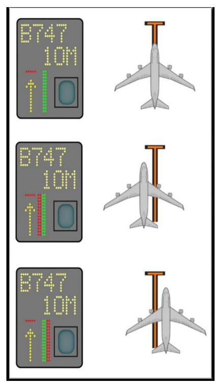
Green light bar illuminates, the aircraft is on centre line. Keep straight ahead.
